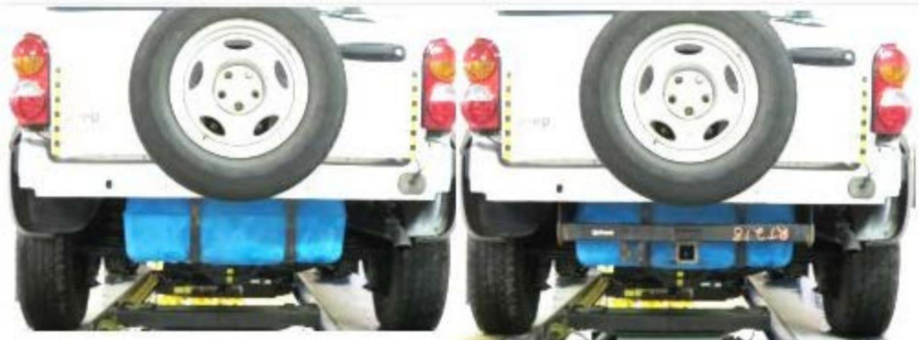
Shown in Yellow: Plastic Fuel Tank Surface that Remains Vulnerable to DIRECT Collision AFTER So-Called "Remedy"
