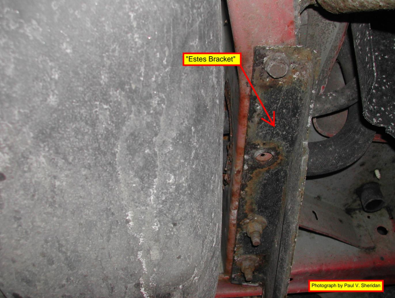
A close-up photograph of a heavily rusted metal bracket on a vehicle chassis. The bracket is a vertical plate with several holes and bolts. A red arrow points from a yellow box containing the text "Estes Bracket" to a specific hole on the bracket. The surrounding area is dark and shows signs of wear and corrosion.
