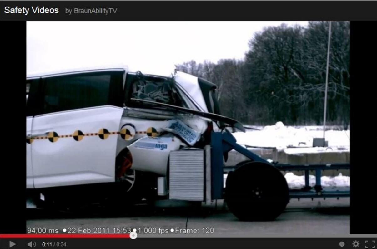
Screenshots of rear intrusion during rear impact crash test by BraunAbility under FMVSS-301 for certification of their wheelchair accessible conversion minivans:
