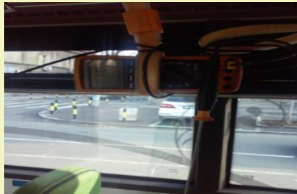
Measuring the temperature of the passenger compartment
