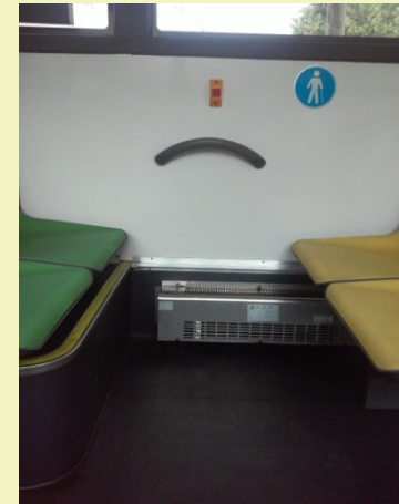
Position radiators for heating
