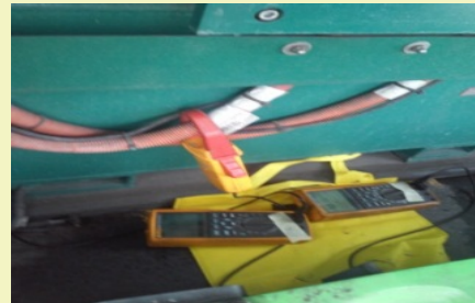
Measurement of voltage and current on a supercondenser
