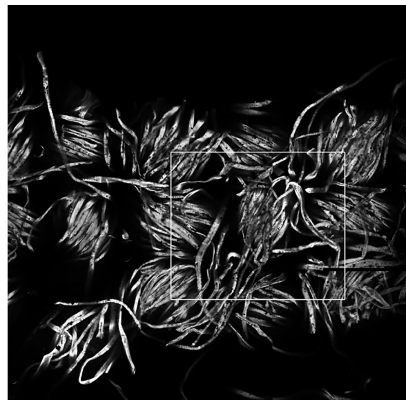
FIG. 2. Slice (number 19, starting at 0) of the confocal image of the fabric. Slice is in the xy plane. The area simulated using LB is enclosed by a white box.
